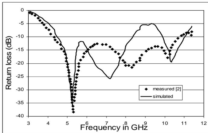
Fig. 13. Return loss (dB) versus frequency plot of a broadband dipole.
