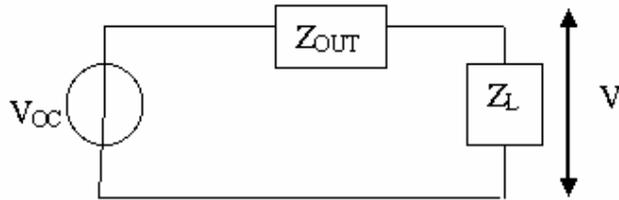
Fig. 2. Thevenin's equivalent circuit diagram of a sensor.
