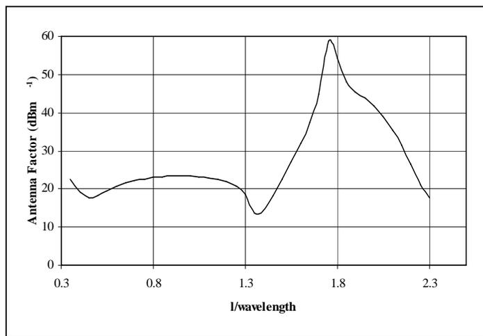
Fig. 4. Plot of antenna factor versus  $L/\lambda$  with radius=0.004 $\lambda$ .
