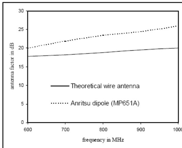
Fig. 5. Comparison of antenna factor of theoretical wire antenna with the Anritsu dipole MP651A antenna.
