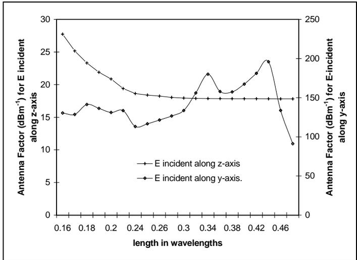
Fig. 9. Antenna factor (dBm<sup>-1</sup>) vs. length in wavelengths of T-shaped antenna.
