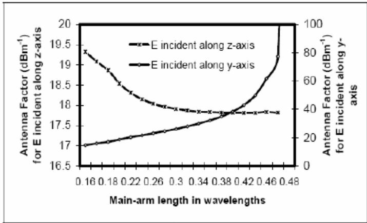
Fig.10. Antenna factor (dBm<sup>-1</sup>) versus length in wavelength of C-shaped antenna.
