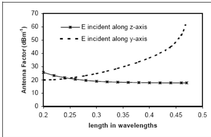
Fig. 8. Antenna factor versus resonant length of inverted L shaped antenna.
