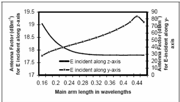
Fig. 11. Antenna factor (dBm<sup>-1</sup>) versus length in wavelengths of I-shaped antenna.
