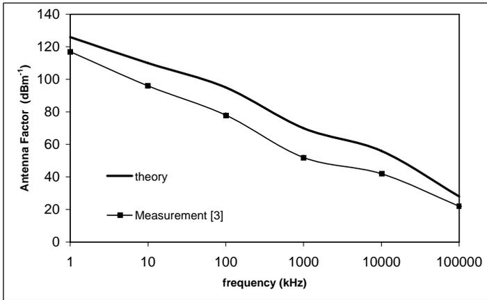
Fig. 12. Antenna factor (dBm<sup>-1</sup>) versus frequency plot of a broadband dipole.
