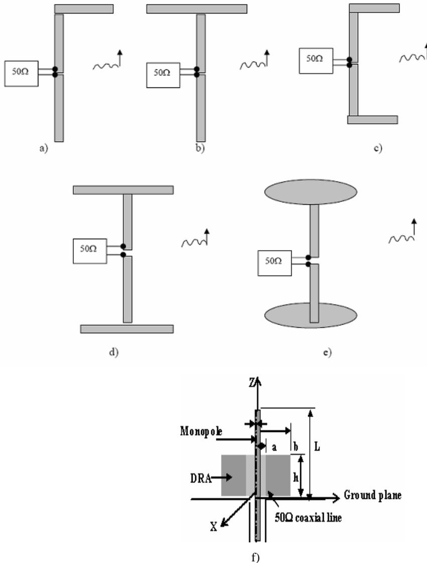
Fig. 1. Different EMI sensors; a) Inverted L antenna; b) T-antenna; c) C-antenna; d) I-antenna; e) Broadband dipole antenna-loaded with circular disc; f) DRA-loaded monopole.
