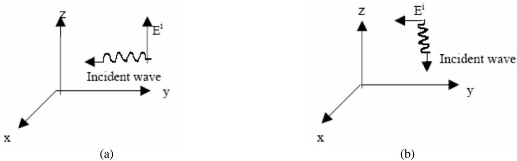
Fig. 3. a) Desired polarization of incident field; b) Cross polarization of incident field.
