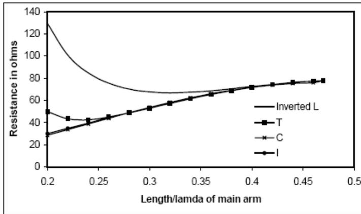
Fig. 7. Resonance resistance in ohm versus corresponding length of the main arms of loaded antennas.
