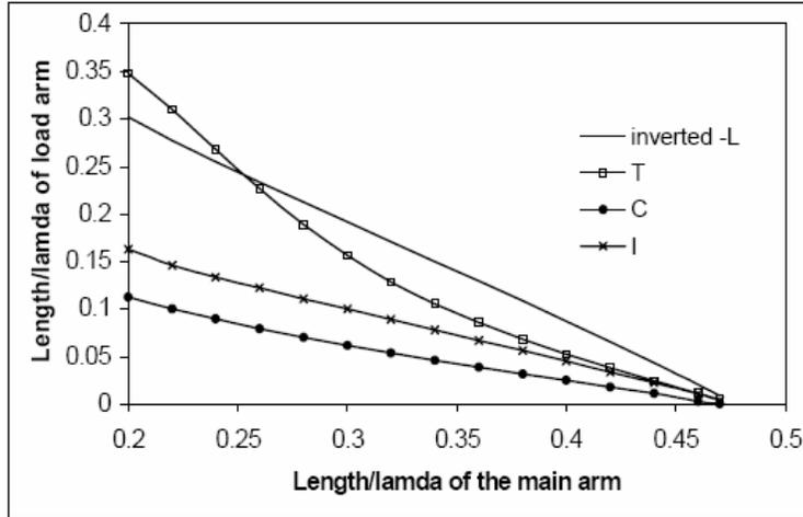
Fig. 6. Length in wavelength of the load arms versus corresponding length of main arms of loaded antennas.
