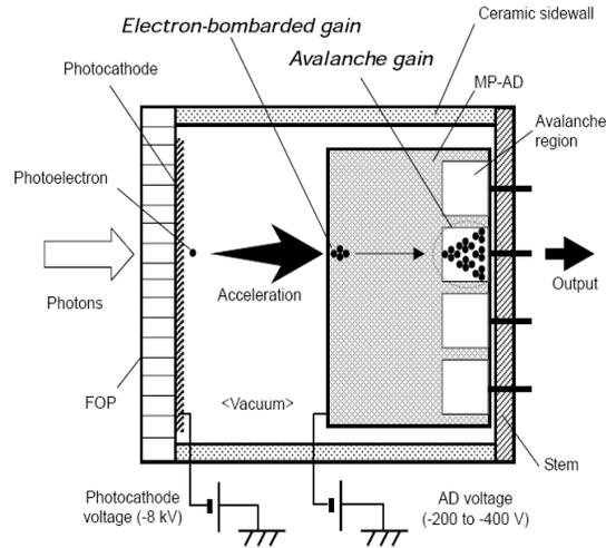
Fig 5: Schematic illustration of the developed HPD.
