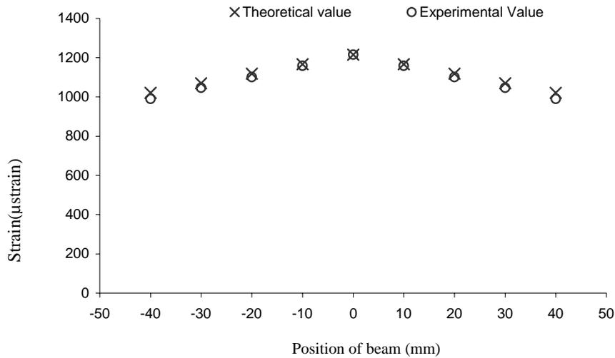
Fig.4. Variation of strain along the beam
