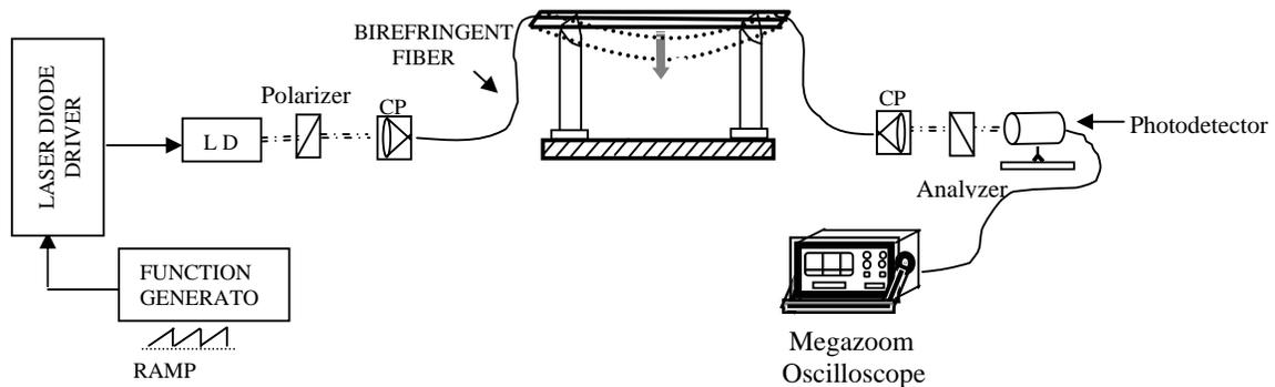
Fig.1. Experimental Set-up: LD-Laser diode, CM-Camera, CP-Optical Coupler, PC- Computer
