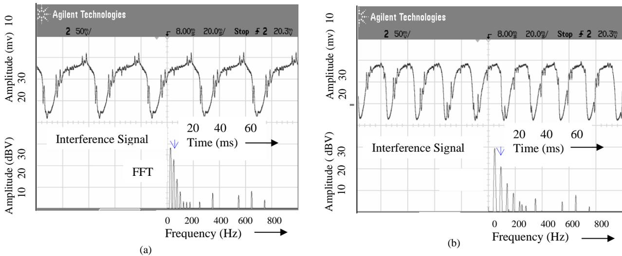
Fig. 2. interference patterns and FFT recorded at different modulating frequencies: (a) and (b) for 1000 gm at 25 Hz, 45 Hz respectively
