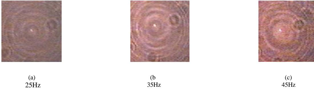
Fig.3. Interference patterns recorded in CCD at different modulating frequency (a) 25 Hz (b) 35Hz (c) 45Hz.
