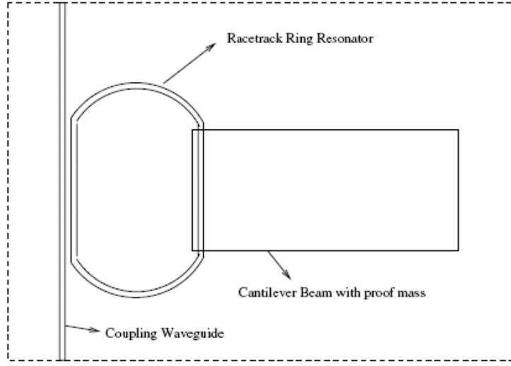
Figure 2. Schematic of the MOEMS vibration sensor with race track resonator
