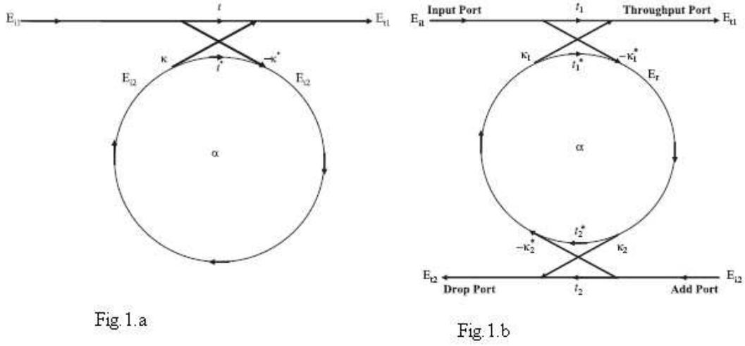
Figure 1. Single Port and Two-port Ring Resonator
