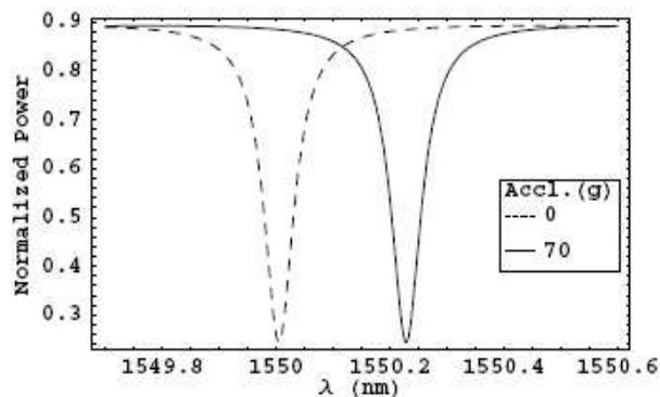
Figure 3. Wavelength shift with and without applied acceleration of 70g for optical MEMS vibration sensor
