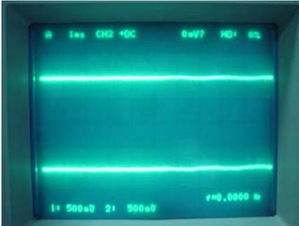
Figure 7. Noise Signal Coupled after EMI Hardening
