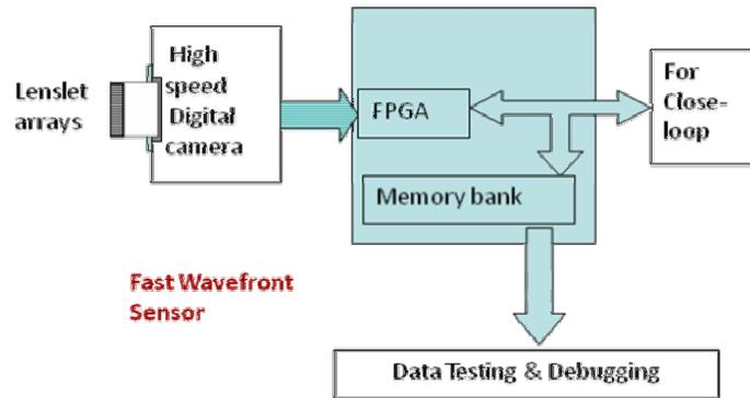
Fig. 1. Design concept of fast SH-WS
