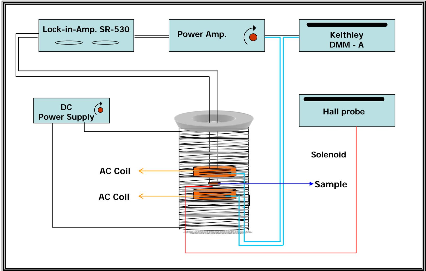
Fig.5. The block diagram of ME set-up working under low fields
