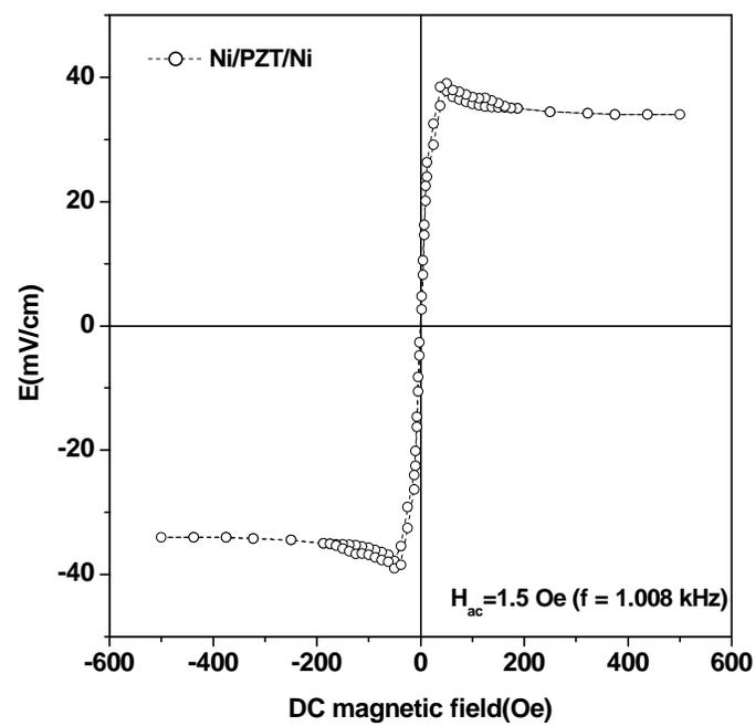
Fig.7. Variation of ME output as a function of dc magnetic field for Ni/PZT/Ni 1:1:1 laminates
