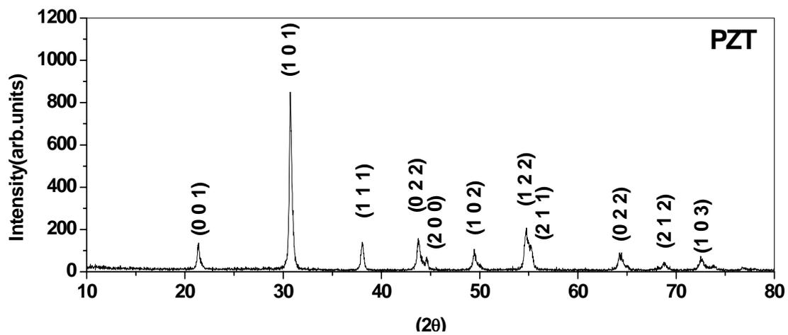
Fig.1. X-ray diffraction pattern of PZT C5 [PZT]
