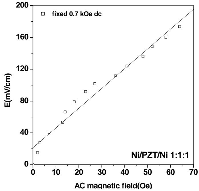
Fig.4. Variation of magnetoelectric output as a function of ac magnetic field for Ni/PZT/Ni 1:1:1 laminates
