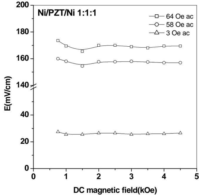
Fig.3. Variation of magnetoelectric output as a function of dc magnetic field for Ni/PZT/Ni 1:1:1 laminates
