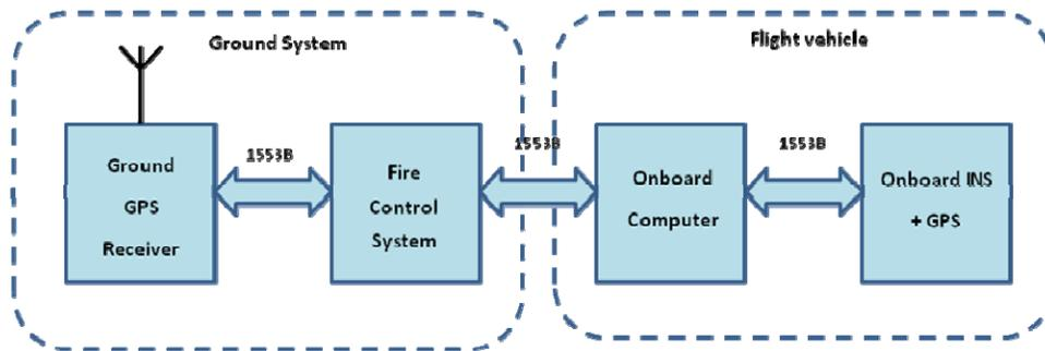
Figure 2 Scheme of uploading the Ephemeris, Almanac, Position and Time data to onboard Receiver
