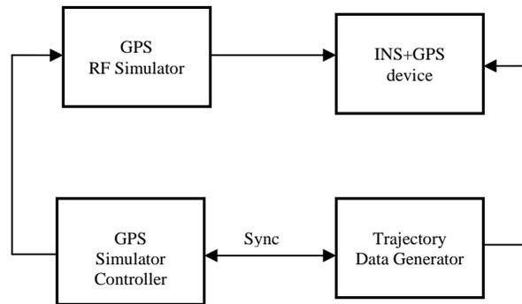
Figure 3. Real Time Flight trajectory Simulation Configuration
