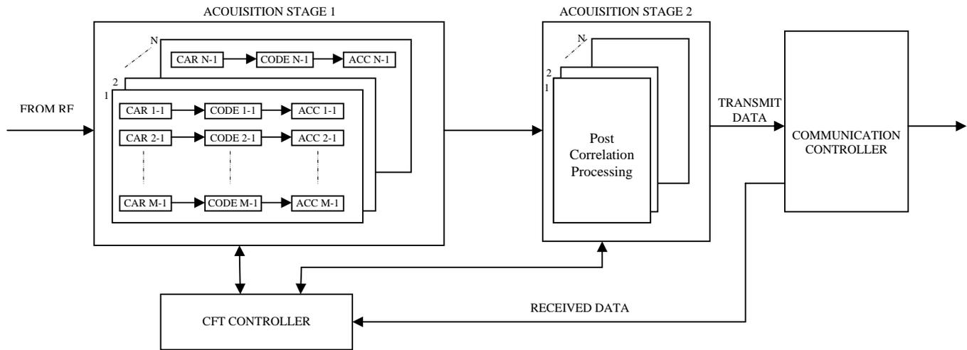
Figure 1. Architecture of Massive Correlators in Fast TTFF Receiver
