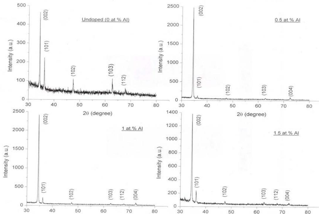
Fig.1: XRD patterns of the typical Al-doped ZnO thin films.
