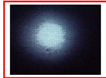
**Fig 3f: TEM<sub>00</sub> mode of 0.6328 μm**
