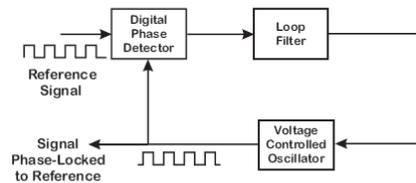
As the resonance frequency keeps varying it develops a phase difference with input drive signal and this difference is used to correct the frequency change.
