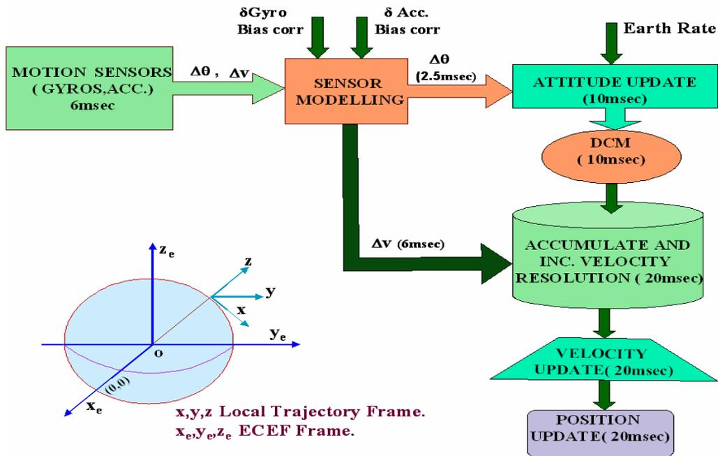
Fig4. Pure Navigation Scheme implemented on ADSP-21060
