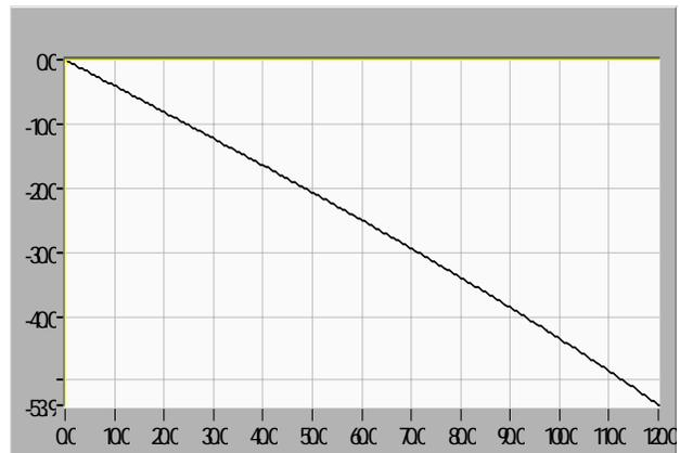
Fig3. Phase response: (Phase in degrees. vs. Frequency in Hz)
