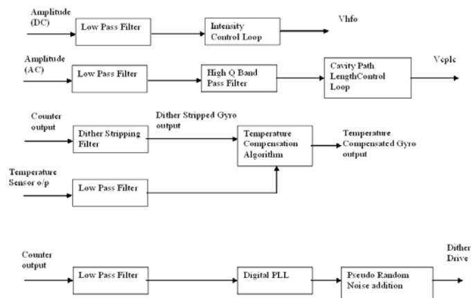
Fig1. Computational blocks of Ring Laser Gyro
