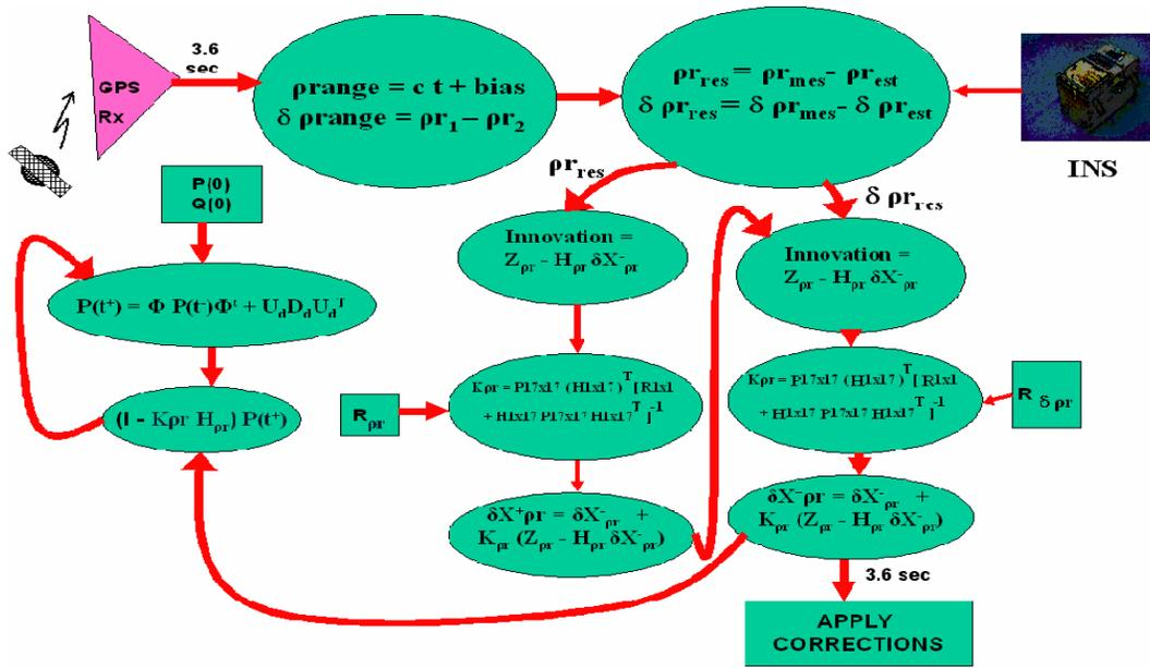
Fig5. Data fusion using Kalman Filter implemented on ADSP-21060
