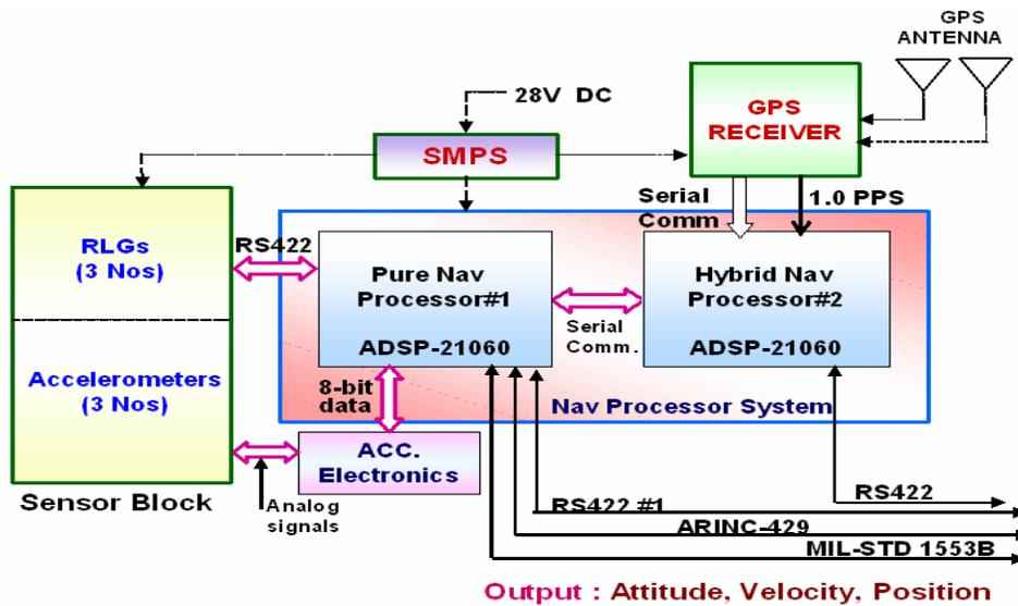
Fig6. Block diagram of Navigation Processor module
