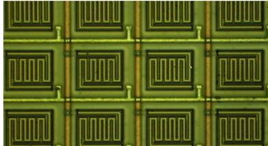
Fig. 1. Photograph of a part of a typical 16x16 microbolometer array
