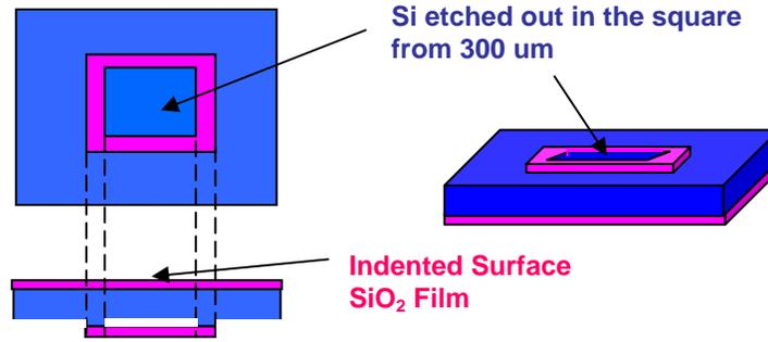
Fig. 1 Silicon etched out from beneath. Silica film on silicon is the indented surface.
