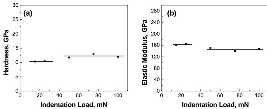
Fig. 3. Variation of (a) Hardness and (b) Elastic Modulus with the indentation load.
