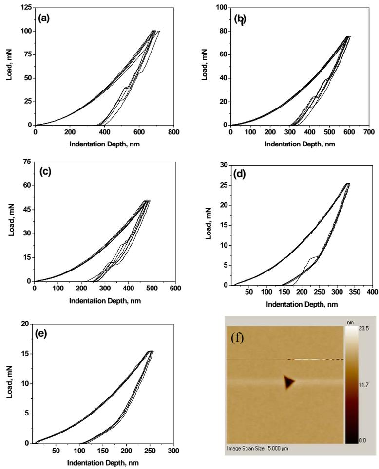
Fig. 2. Load-indentation depth curves for various loads from nanoindentation (a) 100 mN (b) 75 mN (c) 50 mN (d) 25 mN (e) 15 mN (f) AFM image of the residual indent at 50 mN.
