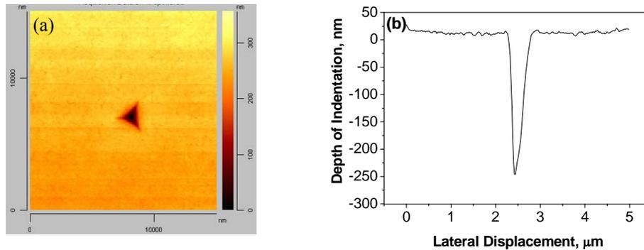
Fig. 6. (a) AFM Image of nanoindentation on silica film. (b) Depth profile of the indentation on silica
