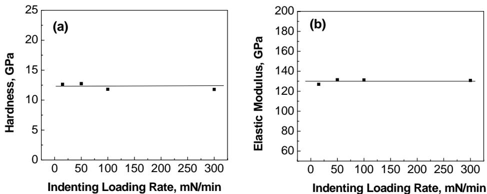
Fig. 4. Variation of (a) Hardness and (b) Elastic Modulus with loading /unloading rate.
