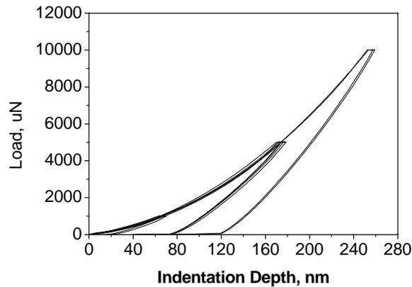
Fig. 5. Load-indentation depth curves for silica film on silicon substrate at various loads
