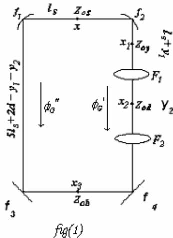
In this arrangement a ring cavity with four 100% reflecting mirrors is considered. Two mirrors  $f_1, f_2$  are spherically concave mirrors and the
