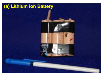
Fig. 1. Assembly details of (a) Pack – 1 (containing only Lithium ion cells) and (b) Hybrid pack (containing Lithium ion cells and Supercapacitor Cells connected in parallel).
