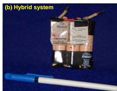
Fig. 1. Assembly details of (a) Pack – 1 (containing only Lithium ion cells) and (b) Hybrid pack (containing Lithium ion cells and Supercapacitor Cells connected in parallel).
