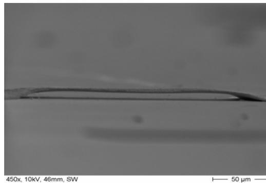
Fig.5. Suspended bridge structure after ashing.
