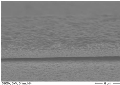
Fig. 4. Surface morphology of the Au electroplated suspended bridge
