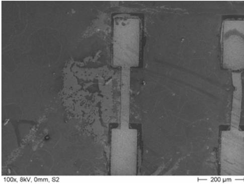
Fig. 2. Top view of Released bridge structure.
