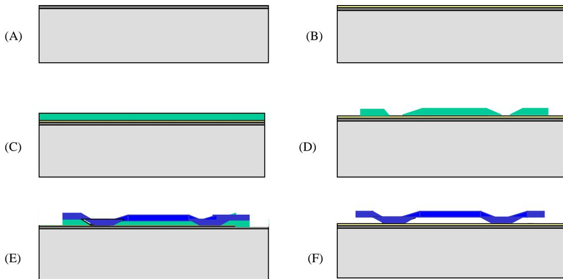
Fig.1. Basic surface micromachining process sequence . (A) Oxidation (B) Metallization (C) Spacer Layer deposition. (D) Anchor patterning with mask (E) Electroplated film deposition (F) Etching of the spacer layer.
