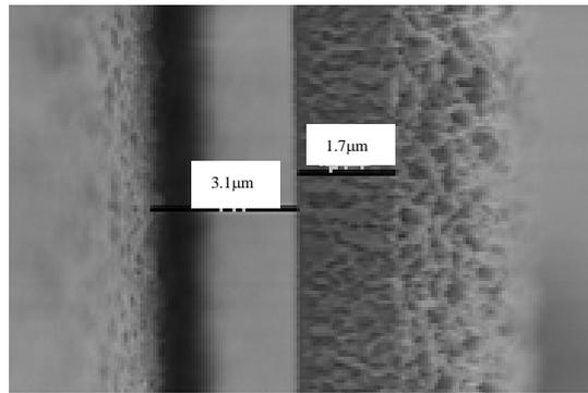
Fig. 3. Crossectional view of the released structure.
