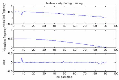
Fig 8. Network output for a 50 KHz Doppler profile
