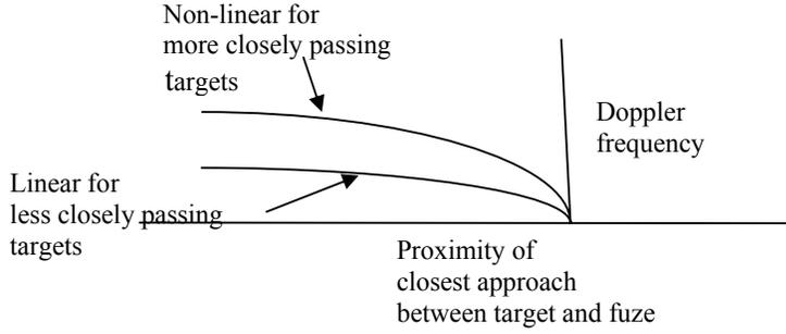
Fig 1. Change in Doppler frequency over time as target passes Proximity fuze
