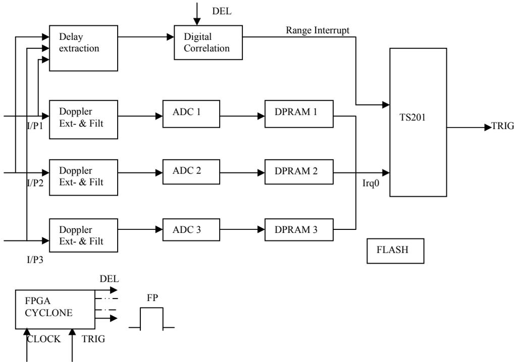
Fig 2. 3-Channel processing DSP Hardware for proximity sensing
