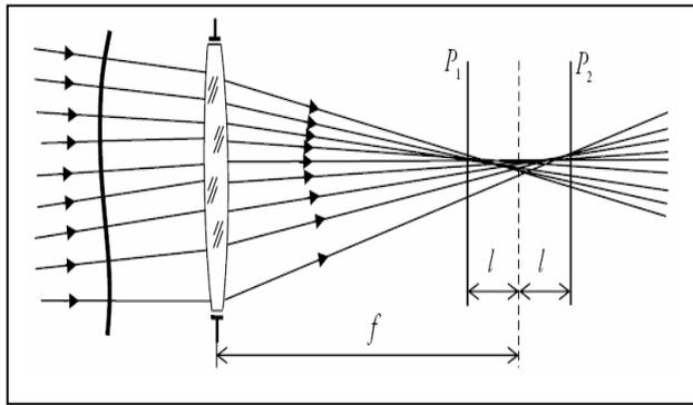
Fig.(1a): Optical-ray diagram for curvature depiction
