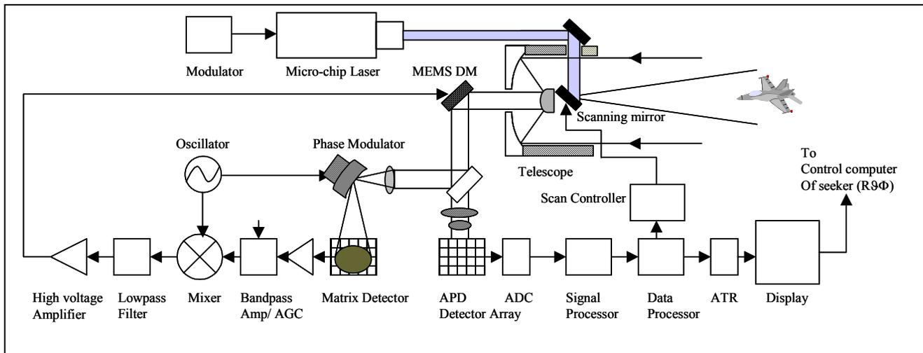
Fig.(3): Opto-electronic schematic of integrated wavefront sensor with Ladar missile seeker
