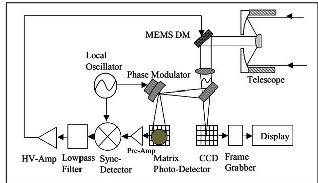
Fig.(1b): Opto-electronic schematic for curvature WFS
