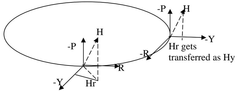
Fig1 Yaw error to Roll error conversion
