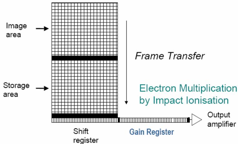
**Fig 4. EMCCD Gain register**
