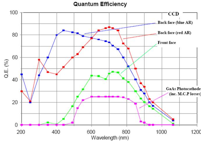
Fig. 2. Comparison of Quantum Efficiencies of Low Light Level CCD sensors
