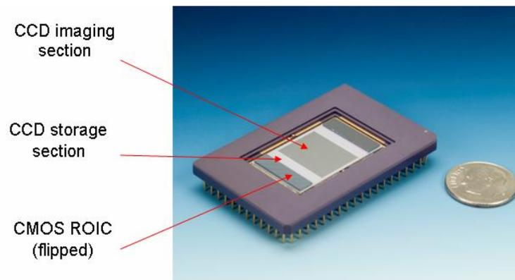
**Fig 6. CCD/CMOS Sensor from Fairchild Imaging, USA**
