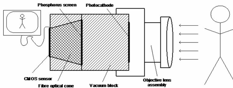
**Fig 5. Pictorial view of Image Intensifier coupled CMOS**
