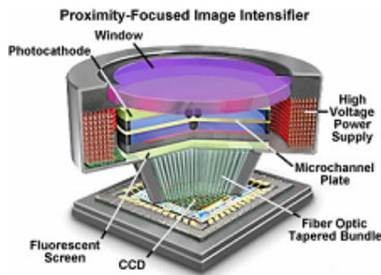
Fig.3 Construction of intensified charge-coupled device
