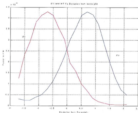
Fig 4. Phase trimmed IF1 and IF2 outputs around boresight.
