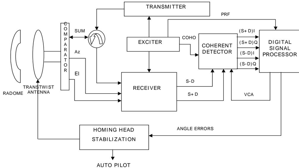
Fig 1. Block Diagram of coherent MMW Seeker.
