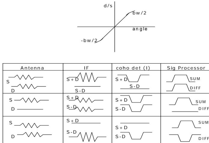
Fig 2. Basic working of the Angle tracking system.
