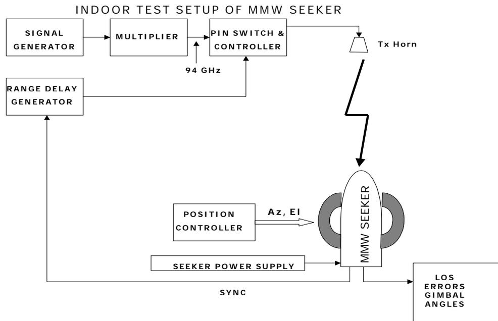
Fig. 3. Indoor test setup of MMW SEEKER
