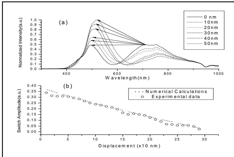
Fig. 3. (a) Spectra at the spectral switch position for different displacements (b) Switch amplitude – vs – displacement
