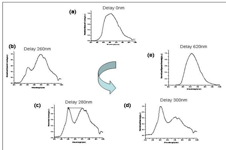
Fig. 2. Normalized spectra measured at the interferometer out put for different path delays
