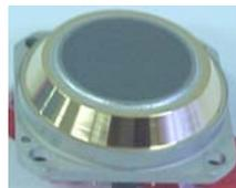
Fig 6. 320x240 Uncooled sensor
