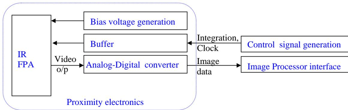
Fig 2. Block diagram of the sensor interface circuit
