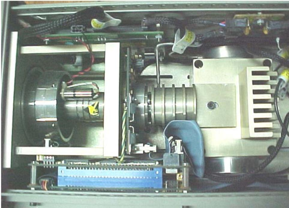
Fig 3 Typical configuration of split stirling cooler based system
