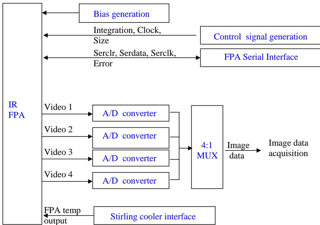
Fig 4. Block diagram of the sensor interface circuit for 320x256 LWIR sensor
