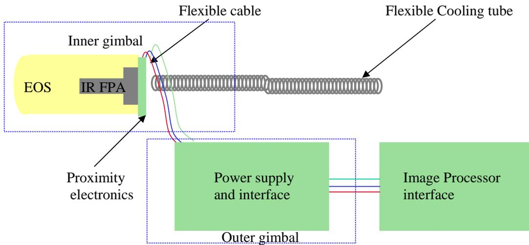
Fig1. Typical seeker configuration with FPA mounted in the inner gimbal
