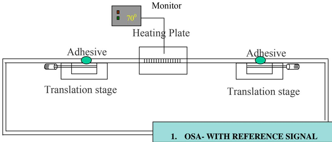
Figure 2: Experimental setup for testing thermal and strain sensitivity of LPGs
