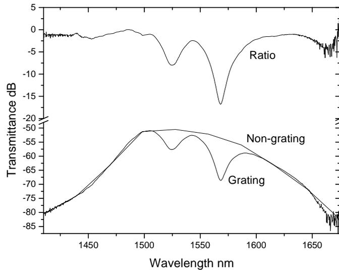
Figure3: Transmission spectrum of the fibre with and without grating
