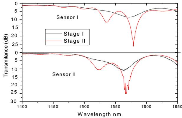
Figure 4: Evolving transmission spectrum of the LPG
