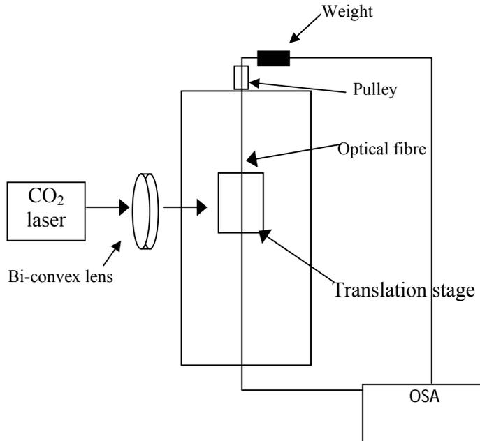
Fig 1: Experimental set up for the writing long period gratings (LPGs)
