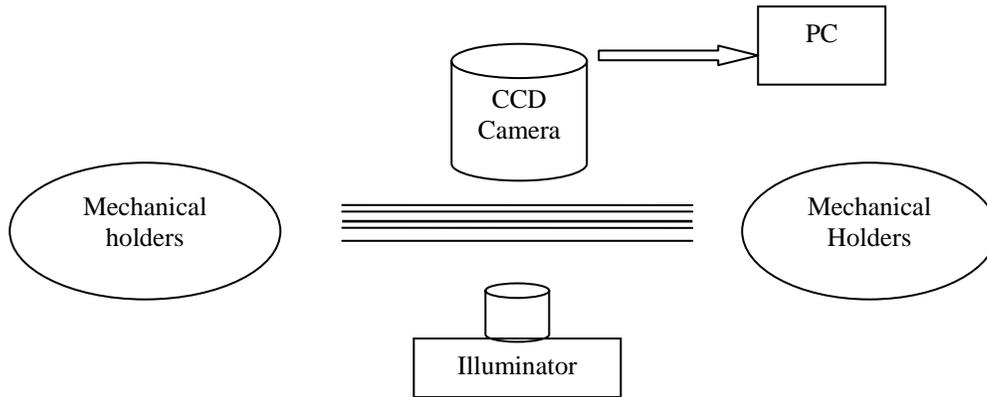
Fig [1]: Birefringent axes alignment assembly
