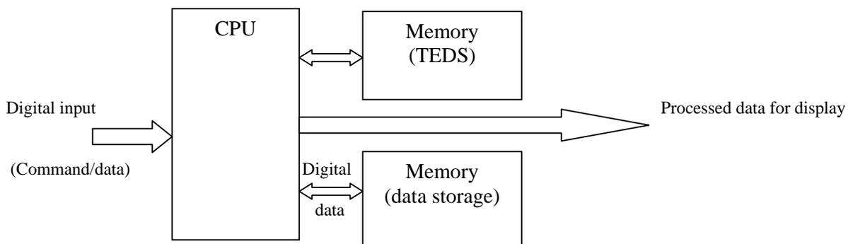
Fig.2 Block diagram representation of Processor Architecture
