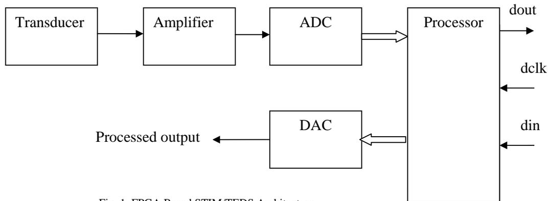
Fig. 1. FPGA Based STIM/TEDS Architecture
