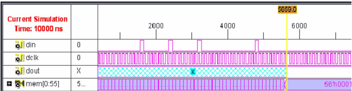
Fig.5 Simulation result for the command : Query TEDS
