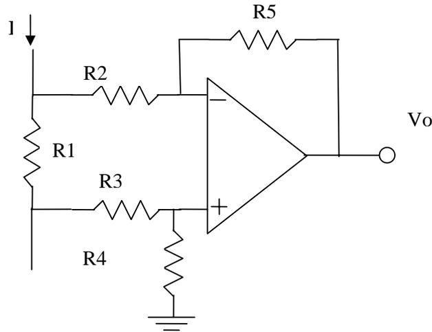
Fig. 3 Differential Amplifier Input Resistive Current Sensor
