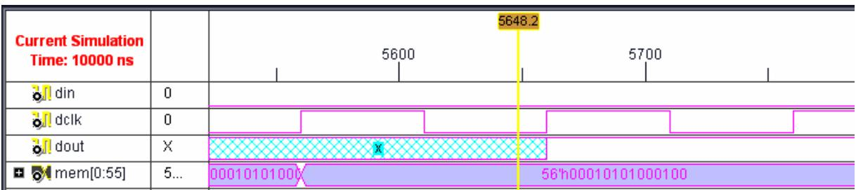
Fig.6 Simulation showing the dout activated after receiving 56 command bits
