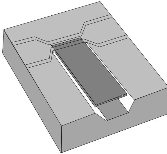
Figure 2. MOEM DC-Cantilever based Vibration Sensor
