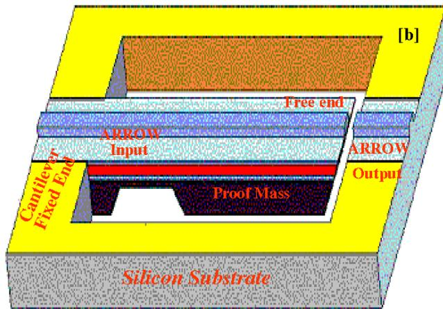
Figure 3. MOEM Waveguide gap Accelerometer
