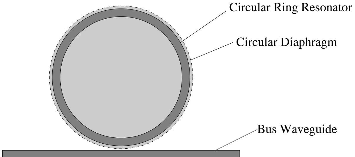
Figure 4. MOEM Ring Resonator Pressure sensor
