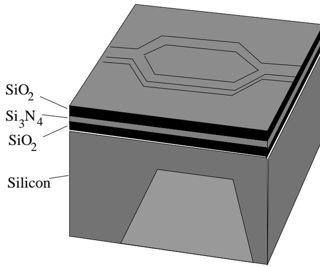
Figure 1. MOEM MZI-Diaphragm based Pressure Sensor
