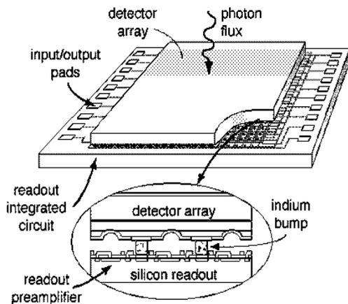
Figure 1(a) Schematic of a hybrid IR FPA. All pixels of the detector array and ROIC are connected via indium bumps.
