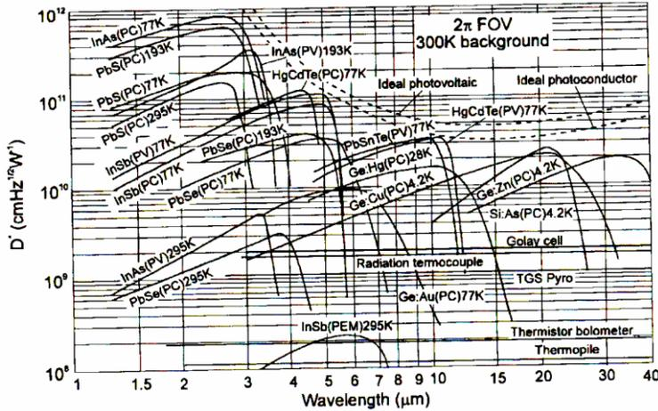
Fig. 2. Comparison of the  $D^*$  of various commercially available infrared detectors when operated at the indicated temperature. Chopping frequency is 1000 Hz for all detectors except the thermopile (10 Hz), thermocouple (10 Hz), thermistor bolometer (10 Hz), Golay cell (10 Hz) and pyroelectric detector (10 Hz). Each detector is assumed to view a hemispherical surround at a temperature of 300 K.
