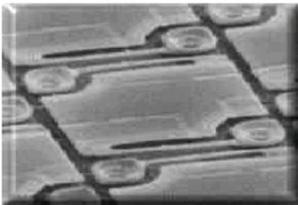
Figure 3: magnified view of an  $\alpha$ -silicon based bolometer detector array.
