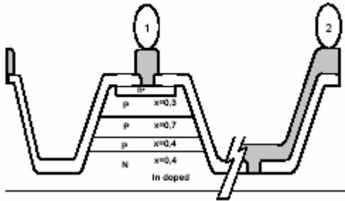
Figure 5 : Schematic cross-section of two-color detector structure
