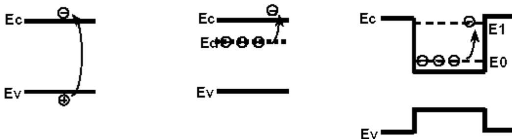
Figure 4: Electron interaction in photon detectors with the incident IR radiation
