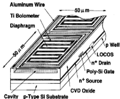
Figure 1(b). Pixel structure for monolithic titanium bolometer IR FPA. Cavities and diaphragms are formed over the ROIC.
