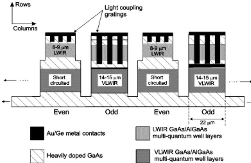
Figure 6. Structure cross-section of the interlace dual-band FPA
