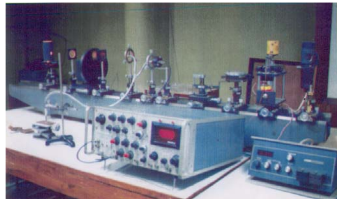
Fig.28 . Experimental setup for in-situ fiber optic colorimetry for detection of corrosion
