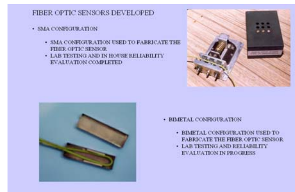
Fig. 35. Microbends in fiber on heating for sensing fire
