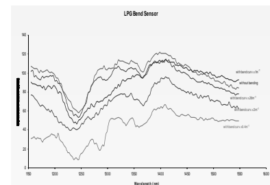
Fig 23 Transmission spectrum of mechanical LPG for different bend curvatures
