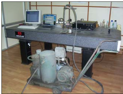
Fig 15. Experimental setup for wind impact of FBG Sensor
