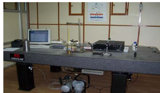
Fig 11. Experimental Setup of Multiplexed FBG Sensors
