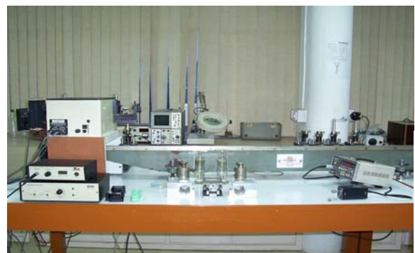
Fig. 30 : Experimental setup of mechanical LPG sensor for refractive index and concentration
