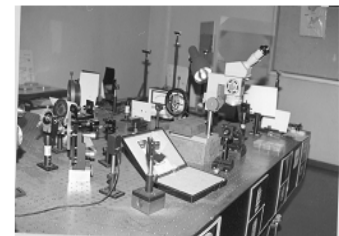
Fig.18 Experimental Setup for EFPI fabrication
