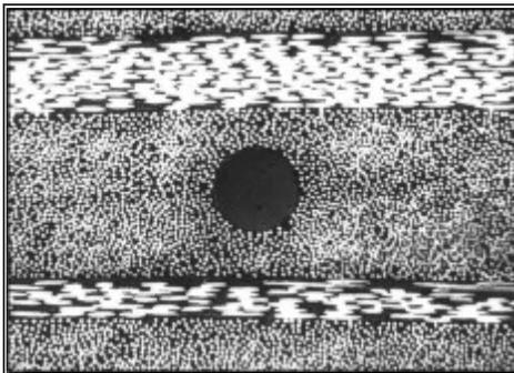
**Magnified cross section of a laminated carbon fiber panel containing an embedded optical fiber sensor (125  $\mu$ m diameter)**
