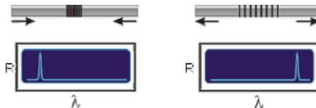
**The diagram above illustrates how the strain applied to a Bragg Grating alters the wavelength of reflected light.**
