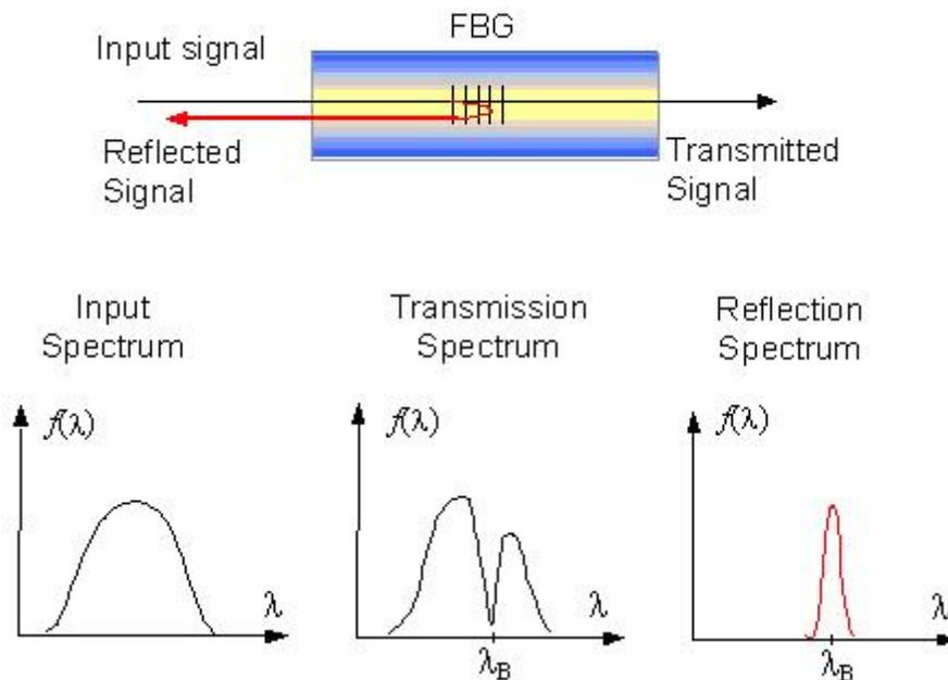
**Fig. 1** Funktional principle of a fiber optic Bragg grating
