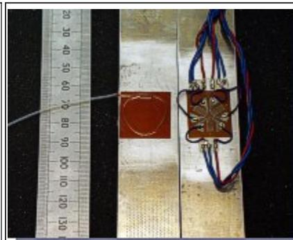
**Comparison of electrical strain gauge rosette (right) and the fiber optic equivalent (left)**
