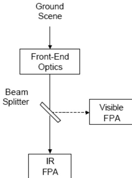
Fig. 5 Fundamental components of dual-band sensor using common front-end optical system [8]
