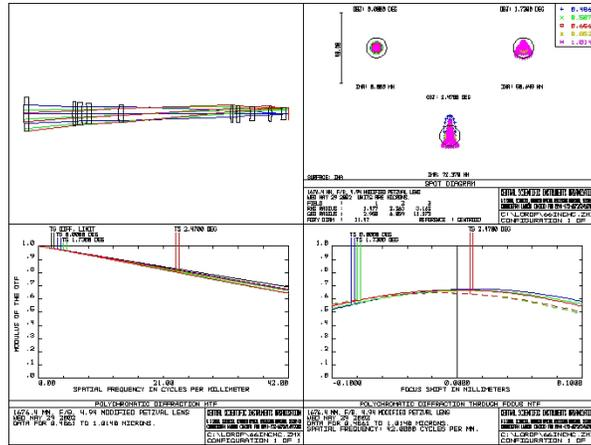
Fig. 3 66-inch (1676.4 mm) focal length f/4 dioptic lens for Itek’s KA-120A Film based LOROP Camera
