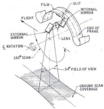
Fig. 1 Basic principle of operation of Minipan [5]
