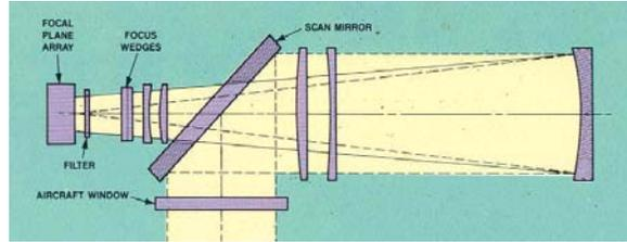
Fig. 4 110-inch (2756 mm) focal length f/5.6 Cata-dioptic lens for Recon's CCD LOROP Camera
