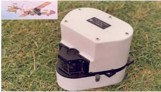
Fig. 2 Minipan Camera D&D by CSIO
