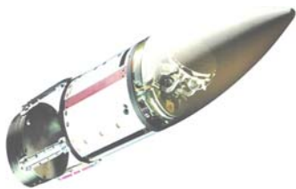
Figure 1: conventional active radar seeker
